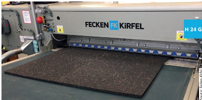
Fig. 6: H 24 G horizontal splitting machine with take-away conveyor for removing the split layers.
