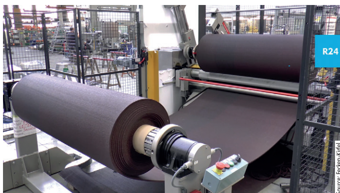
Fig. 10: R 24 bandknife peeling machine – the peeled material sheet is continuously rolled.
