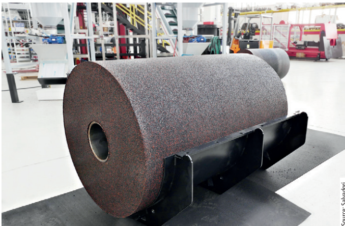
Fig. 4: The standard dimensions for rubber cylinders are a length/width of 1,020 mm, 1,250 mm and 1,520 mm, with a diameter of 1,000 mm. Machines for producing even larger cylinders measuring up to 2,000 mm in width/length and diameter are currently in development.
