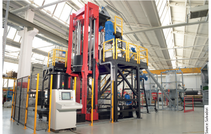
Fig. 3: Salvadori machines turn rubber granulate and binders into cylinders that frequently weigh in at over 1 t.
