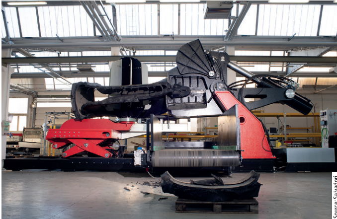
Fig. 2: Salvadori produces equipment for cutting supersize tyres before they are recycled.
