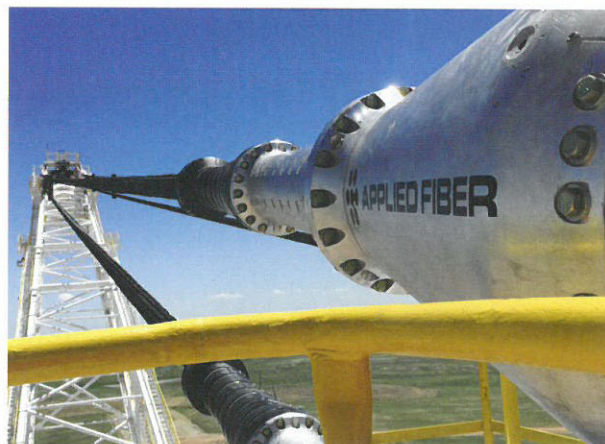
Left: Marion 8200 fibre main boom pendants shown at boom point
