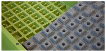
The basic production process is simple: a mixer and a press are the only pieces of equipment you will need if you want to produce moulded goods starting with recycled tire rubber crumb. If, however, you want to industrialize the system to make it a profitable business, you should invest in equipment that allows you to automatize the process and increase your productivity.
